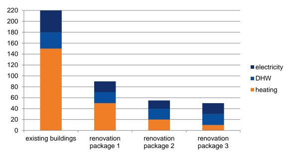
Figure 4. Calculated energy demand of the existing buildings and the three renovation packages in kWh/m<sup>2</sup>a.
