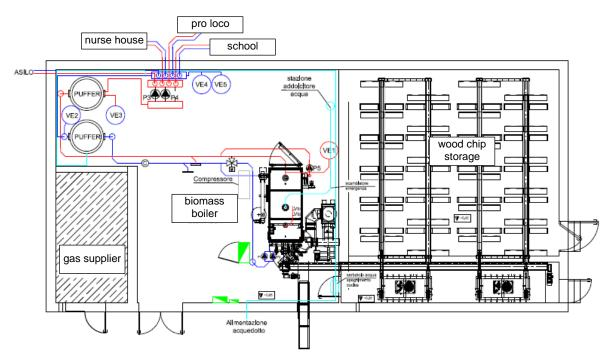
Figure 20. Layout of the thermal plant. Source: technical drawing from as built project, by Comune di Valdastico.
