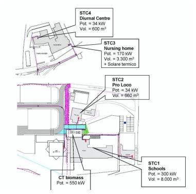
**Figure 21.** The district heating net includes 5 buildings: a CT thermal central station and 4 STC substations. For each building, a label describes the name of the station, the use, the installed power Pot, and the volume Vol. Source: technical drawing from as built project, by Comune di Valdastico.
