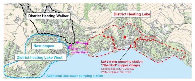
**Figure 50.** Schematic view of the different stages of the district heating networks in Weggis. Source: Corporation Weggis.
