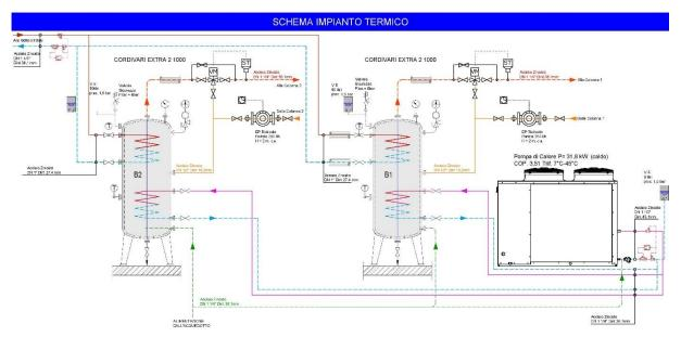
Figure 18. DHW system scheme. Source: ALER- Varese.
