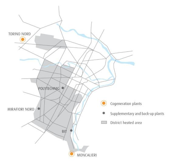
**Figure 24.** Scheme of Turin District Heating Network, showing the two main stations and the supplementary substations for the heated area. Source: Iren Energia S.p.A.
