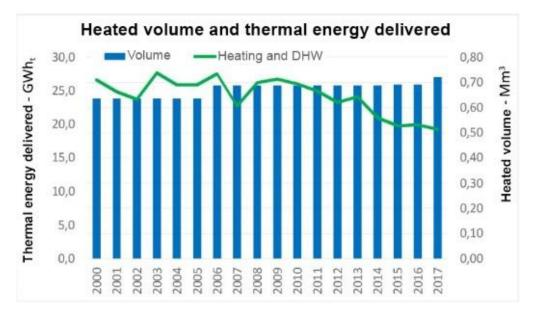
**Figure 13.** Thermal energy supplied to users in GWht for heating and DHW (green line) and volume of housing heated by DH in Mm<sup>3</sup> (blue columns) from the years 2000 to 2017. Source: edited by the authors, based on "Annuario il Riscaldamento Urbano 2018" report by AIRU.
